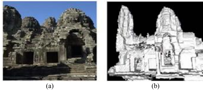
Fig. 2. FLRS result: the object for the experiment (a); the range data obtained (b)
